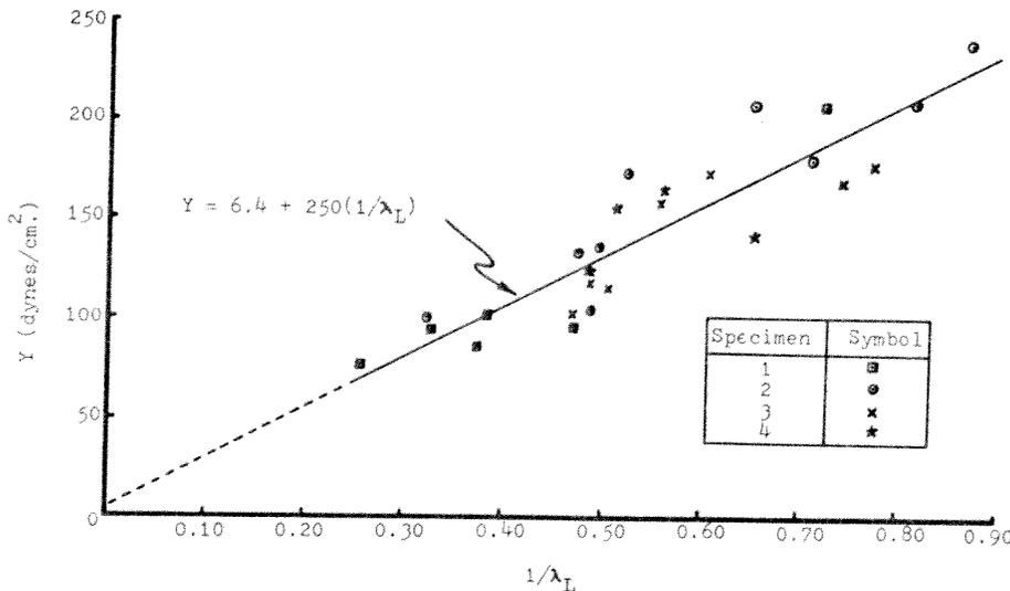
Fig. 3. Simple extension experimental results (Linear regression analysis yields a correlation coefficient = 0.90 and a standard estimate of error = 18.6 dynes/cm<sup>2</sup>).
