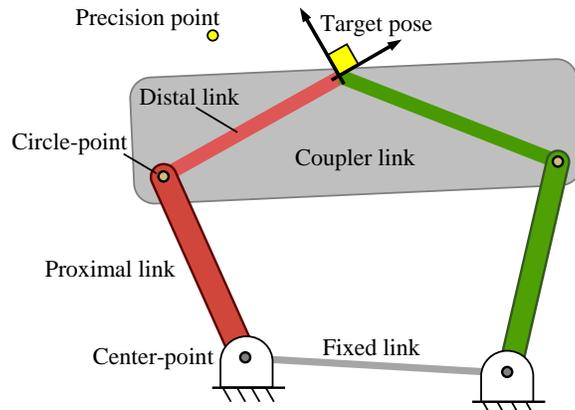
Figure 1: A planar four-bar linkage, achieving a desired pose consisting of target point and orientation. The distal links of two RR dyads are rigidly joined by the coupler.
