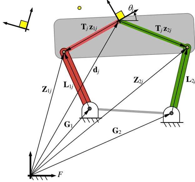
Figure 2: Vector diagram of a four-bar linkage at the  $j^{\text{th}}$  pose. The yellow squares and circle indicate precision poses and a path-point, respectively.
